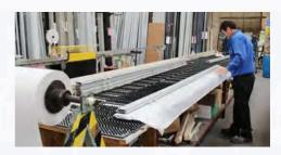
Using fully automated spiral wrappers material is securely packed, this also gives a durable clear protective coating to all bundles.
